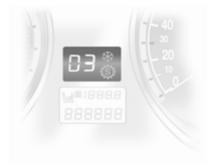
The mode or selected gear is shown in the transmission display.
