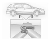
Ensure the jack is positioned correctly with the vehicle jacking points.
