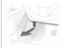
Pull the release lever and return it to its original position.
