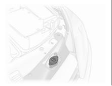
Fill with clean water mixed with a suitable quantity of windscreen washer fluid which contains antifreeze.
