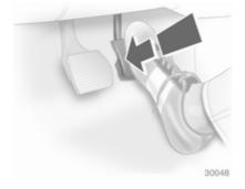
If the accelerator pedal is pressed past the pressure point, the transmission shifts to a lower gear depending on engine speed.
