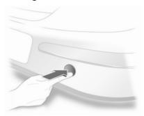
Disengage cap at bottom and remove downwards.
