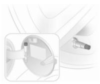
On vehicles with tyre pressure monitoring system, screw the adapter to the valve.
