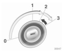
Operate clutch and brake, automatic transmission in **P** or **N**, do not accelerate; for diesel engines, turn the key to position 2 for preheating until control indicator **W** goes out; turn key briefly to position 3 and release key when engine is running. Before restarting or to switch off the
