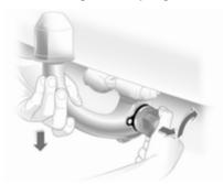
Open the protective flap and turn the key to position  $\widehat{\exists}$  (1) to unlock the coupling ball bar.
