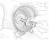
4. Remove the bulb holder with bulb from the reflector.
