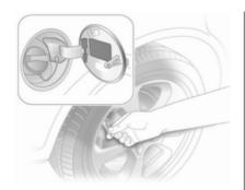
Remove the valve cap key from the fuel filler flap and use it to unscrew the valve cap.
