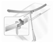
Lift the wiper arm, tilt wiper blade at a 90° to the wiper arm and remove to the side.
