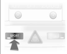
ESP®<sup>Plus</sup> can be deactivated when Sport mode is engaged for high-performance driving:
