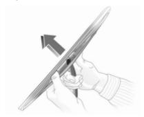
Lift the wiper arm. Disengage the wiper blade and remove.
