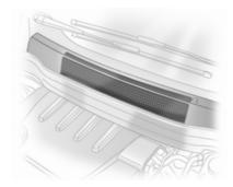
The air intakes in front of the windscreen in the engine compartment must be kept clear to allow air intake. Remove any leaves, dirt or snow.
