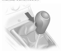
Reverse: with the vehicle stationary, wait 3 seconds after depressing clutch pedal and then pull up the button on the selector lever and engage the gear.
