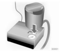
If the prescribed tyre pressure is not obtained within 10 minutes, remove the tyre repair kit. Move the vehicle one tyre rotation. Reattach the tyre repair kit and continue the filling procedure for 10 minutes. If the prescribed tyre pressure is still not obtained, the
