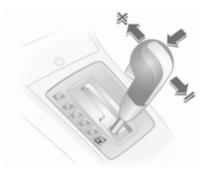
Move selector lever out of position **D** towards the left and then forwards or backwards.
