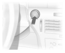
The electronic key must be inside the vehicle. Operate clutch and brake, automatic transmission in **P** or **N**, do not accelerate, for diesel engines, press the button briefly to start preheating, move the steering wheel slightly to release the steering wheel lock, wait until control indicator  $\mathfrak{W}$  goes out and then press button for 1 second and release when the engine is running.
