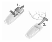
If the radio remote control also fails, the driver's door can be locked or unlocked with the emergency key contained in the electronic key: press locking mechanism and remove the cap by applying light pressure. Push the emergency key outwards over the detent and remove
