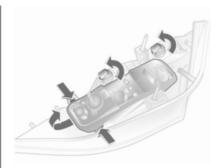
Disengage sockets by turning and remove. Press locking tabs on the long sides of the bulb holder outwards; lift bulb holder at front end and remove.
