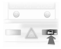
Press the button: the doors are locked or unlocked.
