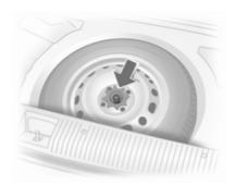
The spare wheel is in the load compartment beneath the floor covering. It is secured in the recess with a wing nut.
