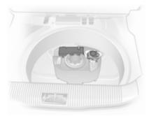
The tyre repair kit is in the stowage compartment under the floor cover in the load compartment.
