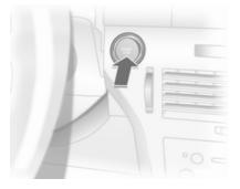
The electronic key must be inside the vehicle. Operate clutch and brake, automatic transmission in P or N, do not accelerate, for diesel engine, press the button briefly to start preheating, move the steering wheel slightly to release the steering wheel lock, wait until control indicator  $\mathfrak{W}$  goes out and then press button for 1 second and release when the engine is running.
