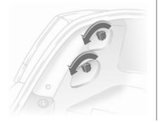
1. Unscrew retaining nuts.
