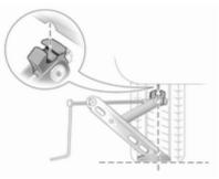
Set the jack to the necessary height before positioning it directly below the jacking point in a manner that prevents it from slipping.
