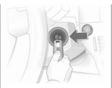
Hold the electronic key at the marked position and press the **Start/Stop** button.
