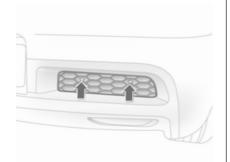
For other models unclip locking tabs downward and pull off the cover upwards.
