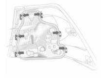
5. Press out six locking catches on the bulb housing and remove bulb carrier.
