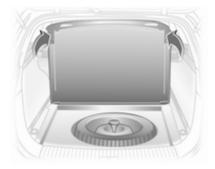
Take adapter and hooks from the rails in the load compartment walls. Raise the rear lashing eyes and lift the floor cover to the vertical position so that it rests on the roof lining. When closing, guide the lashing eyes through the slots in the floor cover. Vehicles with cargo box: removal ⋄ 73.
