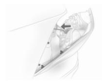
Press tail lights back, holding the bulb housing from the outside. Remove plug from bulb carrier.
