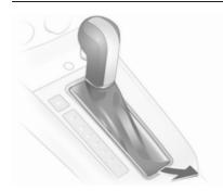
If the battery is not the cause of the fault, release selector lever:
