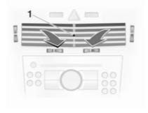
To open vent, turn the adjuster wheel to I.
