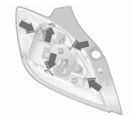
Unscrew the three screws using a screwdriver. Press the locking tabs on the outside of the bulb holder inwards and remove the bulb holder.
