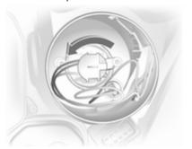
3. Rotate left bulb holder and disengage.
