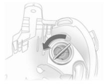
2. Rotate bulb holder anti-clockwise and disengage.
