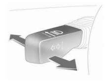
Headlight flash = Pull lever High beam = Push lever
