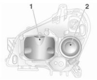
Headlamps have separate systems for low beam 1 (inner bulbs) and high beam 2 (outer bulbs).
