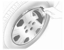
1. Pull off the wheel cover with the hook. Vehicle tools \$\Display\$ 184.
