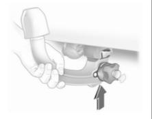
Insert the tensioned coupling ball bar in the opening and push firmly upwards until it audibly engages.
