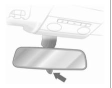
Swivel the lever on the underside to reduce dazzle.
