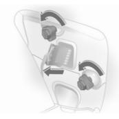
3. Loosen fastening nuts with wheel bolt wrench and unscrew by hand. Vehicle tools
