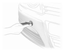
Disengage the cover at the bottom and remove downwards.
