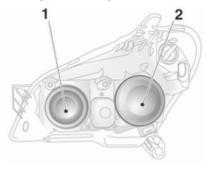
Headlights have separate systems for high beam 1 (inner bulbs) and low beam 2 (outer bulbs).
