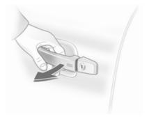
Pull a door handle or press the button under the tailgate moulding.
