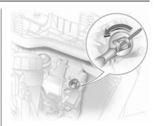
If the vehicle must be moved out of the flow of traffic, disengage the clutch as follows (for vehicles with 5speed manual transmission automated only):
