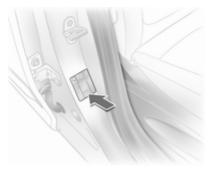
The identification plate is located on the front right door frame.
