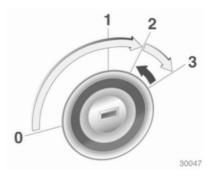
Turn key to position 1. Move the steering wheel slightly to release the steering wheel lock. Operate clutch and brake, automatic transmission in **P** or **N**, do not accelerate; for diesel engines, turn the key to position 2 for preheating and wait until control indicator  $\mathfrak{W}$  goes out; turn key to 3 and release key when engine is running.
