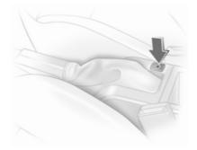
An external audio source such as a portable CD player can be connected using a 3.5 mm jack plug via the AUX input.
