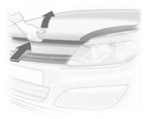
Lift the safety catch upwards and open the bonnet.
