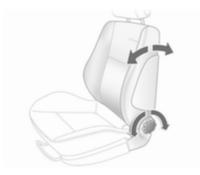
Turn handwheel. Do not lean on seat when adjusting.
