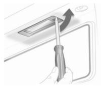
Insert a screwdriver in the housing, press to the side and release spring.
