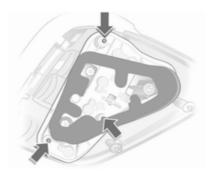
4. Unscrew the three screws with a screwdriver and remove the bulb holder. Vehicle tools ▷ 184.
