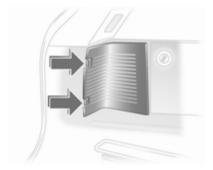
1. Disengage cover by pressing retaining lugs and remove.
