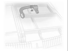
In Saloons, the coupling ball bar is in a pouch, fastened in the load compartment cargo box with a strap. In Station wagons, the coupling ball bar is fastened with a strap in a compartment in the spare wheel well of the load compartment.
