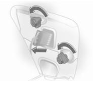
3. Loosen fastening nuts with wheel bolt wrench and unscrew by hand. Vehicle tools
