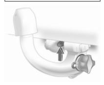
Lock the coupling ball bar by turning the key to position  $\[ \odot \]$  (2). Remove the key and close the protective flap.
