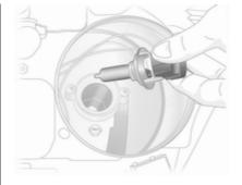
4. Detach bulb from bulb holder and renew the bulb.
