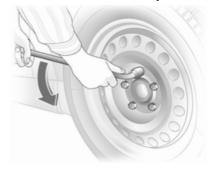
Install the wheel wrench ensuring that it locates securely and slacken each bolt by half a turn.
