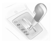
The selector lever can only be moved out of **P** or **N** when the ignition is on and the foot brake is depressed (selector lever lock).
