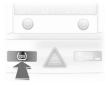
After tyre pressure correction or wheel change, the system must be initialised: Switch on the ignition,
