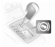
When the selector lever is in the P or N position, control indicator (S) in the gear indicator strip illuminates red when the selector lever is locked. If the selector lever is not in the P position when the ignition is switched off, control indicator (S) and P in the gear indicator strip flash.
