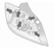
Remove seal from the fastening bolt. Press the locking tabs on the outside of the bulb holder outward and remove the bulb holder.
