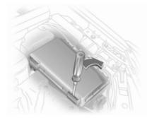
Insert a screwdriver into the opening as far as it will go and tilt it sideways. Open the cover upwards and remove.
