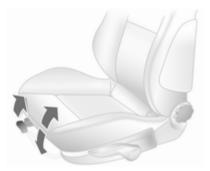
Pull lever, adjust inclination by shifting body weight. Release lever and audibly engage seat in position. Seat adjustment ₱ 49, Seat position ₱ 49.
