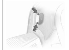
Release the bolts behind the cover using a conventional bolt wrench, and remove.
