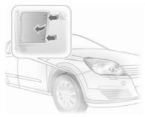
The bulbs of the front outer lights are replaced through openings in the front wheel housing: turn wheels in a way that allows access, release catch and remove cover.
