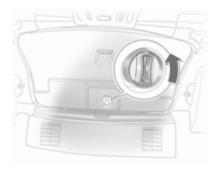
From the interior, turn the rotary knob on the inside of the boot lid anticlockwise, this unlocks the boot lid and opens it slightly.
