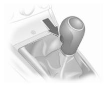
To engage reverse, with the vehicle stationary wait 3 seconds after depressing the clutch pedal and then pull up the button on the selector lever and engage the gear.
