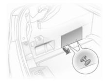
To open, pull the two knobs, remove the clips and fold the cover upwards.
