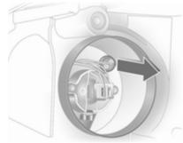
3. Withdraw parking light bulb holder from reflector.
