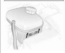
When the cooling system is cold, the coolant level should be just above the **KALT/COLD** mark. Top up if the level is low.
