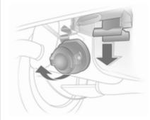
Fold down the socket. Remove the sealing plug from the hole for the coupling ball bar and stow it in the load compartment.
