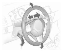
Unlock lever, adjust steering wheel, then engage lever and ensure it is fully locked. Do not adjust steering wheel unless vehicle is stationary and steering wheel lock has been released.
