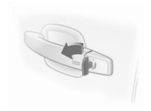
The emergency key can only lock or unlock the driver's door. Unlocking the entire vehicle ♀ 25. On vehicles with anti-theft alarm system, the alarm may be triggered when the vehicle is unlocked. Deactivate the alarm by switching on the ignition.
