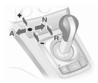
Always move the selector lever in the appropriate direction as far as it will go. Upon release, it automatically returns to the centre position.
