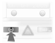
After a wheel change, the system must be initialised: inflate the tyres to the prescribed pressure, switch on the ignition, press and hold the **DDS** button for approx. 4 seconds, control indicator (!) flashes three times.
