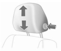
Press release button, adjust height, engage.
