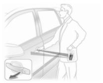
When in possession of the electronic key, simply pulling the door handle will unlock the vehicle and open the door. To open the tailgate, press the button under the moulding.
