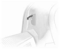
To replace bulbs, fold up cover in load compartment after twisting the catch.
