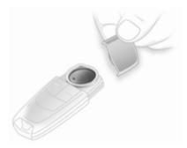
To replace the battery, press the locking mechanism and remove the cap by applying light pressure. Press the cap on the other side outwards.
