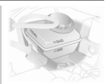
The brake fluid level must be between the **MIN** and the **MAX** marks.
