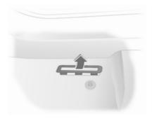
The Vehicle Identification Number is stamped on the identification plate and on the floor pan, under the floor covering, visible under a cover.
