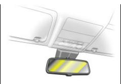
Automatic anti-dazzle interior mirror \* Dazzling at night is reduced automatically.
