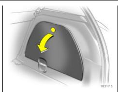
The tyre repair kit is located in the compartment to the right in the luggage compartment.
