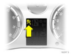
Control indicator 2, front passenger airbag systems which can be deactivated When the ignition is switched on, 2 flashes for approx. 15 seconds. The airbag systems for the front passenger can only be activated or deactivated during this time. LEDs illuminated in the button 2 and illumination of the control indicator 2 indicate deactivated airbags, but if the LEDs and control indicator 2 are not on, the airbags are activated.
