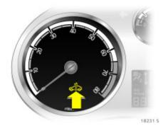
Control indicator for immobilizer औ Control indicator औ illuminates briefly when the ignition is switched on.
