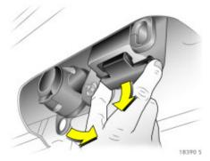
Fold down socket. Pull sealing plug out of coupling ball bar opening. Place cover and coupling ball bar in luggage compartment.
