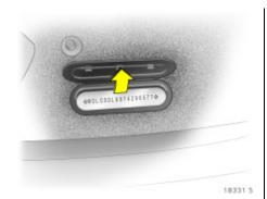
The vehicle identification number is stamped on the identification plate and on the right side of the floor of the vehicle under a cover between the front door and the seat.
