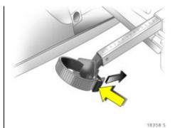
Insert the strap retainer and pull tightly downwards as far as possible.
