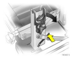
Disengage the locking lever on the diagonal support and fold both pedal crank recesses down.
