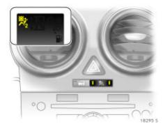
The airbag systems for the front passenger are now deactivated. To indicate this, both LEDs in the button  $\frac{2}{3}$  and the control indicator  $\frac{2}{3}$  remain on when the ignition is on.
