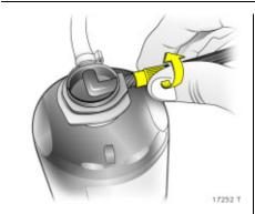
2. Unwind the air tube from the holder and screw onto the sealant bottle connector.
