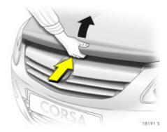
Lift the safety catch upwards and open the bonnet.
