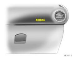
The front passenger airbag system **\*** can be recognised by the text **AIRBAG** above the glove compartment.
