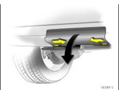
Fitting the coupling ball bar Push both bolts inwards and remove the cover on the bumper.
