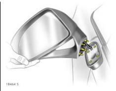
For the safety of pedestrians, the exterior mirrors of the Corsa OPC are released from the holder if they are bumped. Fit mirror housing to holder with latching lugs and engage by striking gently.
