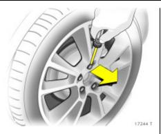
Alloy wheels \*: Disengage the wheel bolt caps with a screwdriver and remove. Protect the wheel by inserting a soft cloth between the screwdriver and ally wheel.
