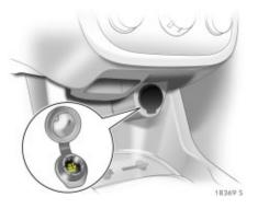
Electrical accessories connected to the socket must comply with the electromagnetic compatibility requirements laid down in DIN VDE 40 839, otherwise vehicle malfunctions may occur.
