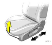
To adjust front seat leg room: Pull handle, slide seat, release handle
