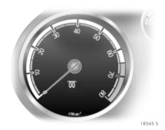
The control indicator  ${\mathfrak W}$  goes off as soon as the self-cleaning operation is complete.
