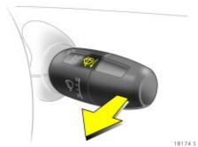
Windscreen washer system Pull stalk towards steering wheel. Screen wash is squirted onto the screen and the wipers move back and forth a few times.
