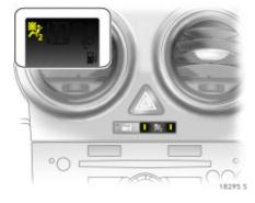
In the event of a fault in the airbag systems, the LEDs flash in the button ½ for switching off the airbag systems ¾, the control indicator ½ also illuminates.
