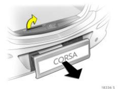
Extend Flex-Fix system Open the tailgate \$ 36.
