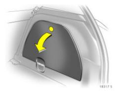
The towing eye is in the luggage compartment, on the right beneath the cover.
