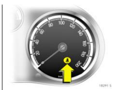
Control indicator & indicating that driver's seat belt has not been fastened When the ignition is switched on, the control indicator & comes on for approx. 15 seconds.
