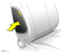
The side airbag system  $\divideontimes$  is identified by the covers on the outboard sides of the front seat backrests.
