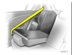
Disengage the backrest (single or split \*) using the release lever and fold it down onto the seat cushion.
