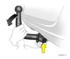
Inserting the coupling ball bar Insert the tensioned coupling ball bar in the housing and push firmly upwards until it audibly engages.
