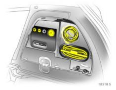
Remove the sealant bottle and holder with the air tube from the compartment.
