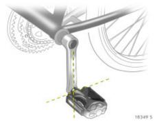
Prepare the bicycle for attachment Rotate the left pedal (without a chain leaf) vertically downwards. The pedal on the left pedal crank must be horizontal.
