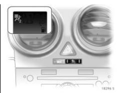
The airbag systems for the front passenger are now activated. To indicate this, LEDs in the button 2 and the control indicator 2 must not be on.
