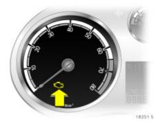
Control indicator ( for exhaust Illuminates when the ignition is switched on and during the start attempt. Goes off shortly after the engine starts running.
