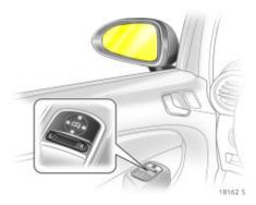
Setting with four-way switch in version with electronic window operation
