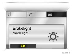
If there is a fault in the lighting system, the respective location of the fault is displayed as text, e.g.:
