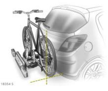
Align the bicycle in the longitudinal direction of the vehicle: Loosen the locking screw on the crank bearing fixing a little \$ 177, Fig. S 14629.
