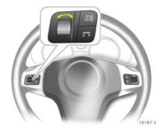
Selection using left adjusting wheel on steering wheel **%**: Rotate and press knurled wheel.
