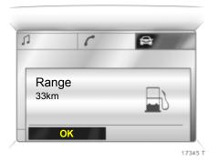
If the fuel in the tank will allow less than 50 km of travel, the message Range appears in the display.
