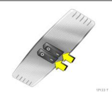
Courtesy lamps and rear reading lamps \* Operated with switch (I = on, 0 = off, centre = automatic interior light).
