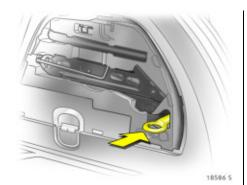
The towing eye is located in a recess.
