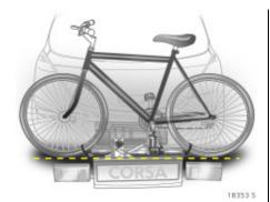
Both bicycle tyres must be in the wheel recesses. In order to prevent damage, neither the pedal bearing housing on the bicycle nor the pedal crank must not be touching the pedal crank recess.
