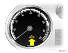
Control indicator & for engine electronics Illuminates for a few seconds after the ignition is switched on.
